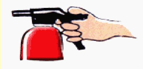
**7** **SQUEEZE**... the handle. This releases the extinguishing agent.
